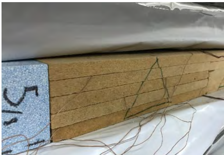
Figure 69 : Separated specimen installed in the GHP apparatus with thermocouples between the layers. The sides are insulated with EPS. The whole specimen is sealed on all sides with a vapor barrier.
