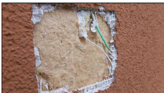
Figure 44: Open measuring position P at variant N 2.6 (dark render) after the test period. No fungal mycelium visible.
