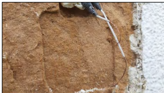
Figure 49 : Opened measuring position P at variant N 2.8 (bright-coloured render) after the test period. No fungal mycelium visible.
