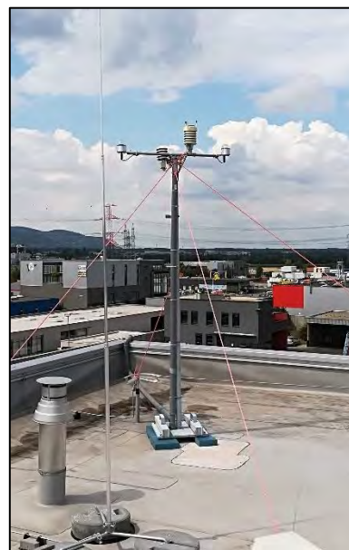
Figure 14 : Weather station on the roof of the ACA in Stetten
