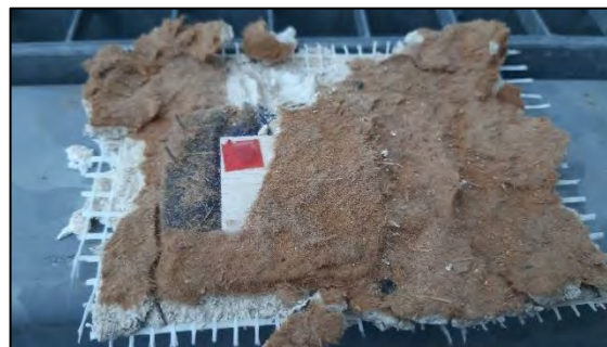
Figure 50 : Removed render layer of variant N 2.8 (bright-coloured render) with Balsa sensor and wood fibre residues. No fungal mycelium visible.
