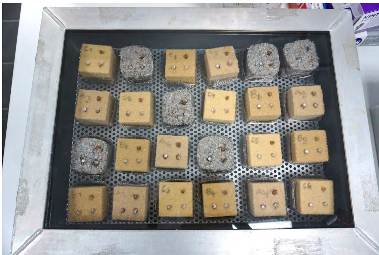
Figure 27 : Incubation unit with inoculated specimens. The tray filled with salt solution or distilled water is located under the metal grid.
