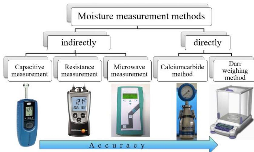
Fig. 16 Common devices for measuring moisture in constructions
