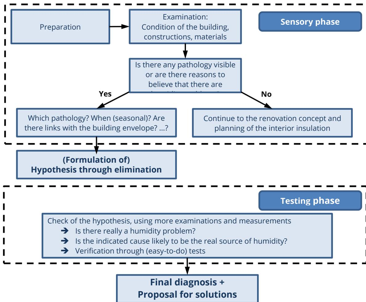
Fig. 3 Overview of the on-site investigation process
